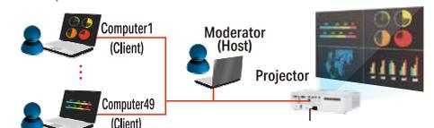
\*To secure better performance, a wired network is preferable. Required to install the LiveViewer software on all the computers. The functions are supported by LiveViewer (Windows® application) only.
