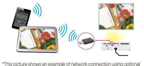
\*This picture shows an example of network connection using optional wireless adapter.
